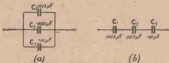
Fig. 3.—Condensers in series or parallel are useful for many purposes.
