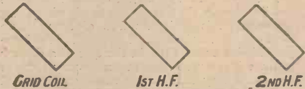
Fig. 2.—A popular method used to avoid coupling between the H.F. coils.
