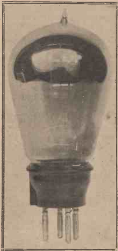
A typical valve with a low amplification ratio.
