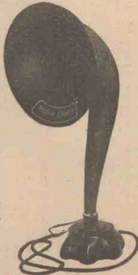
For best results the horn must not be less than a certain length.
